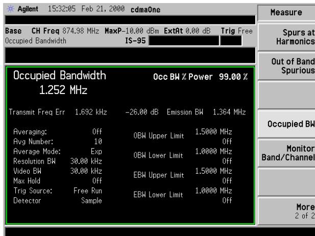
Figure 3-20 Numeric +Parameters View with a Good cdmaOne Signal
